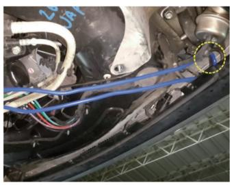
Locate the vacuum source where is on the rear chassis as indicated, the solenoid of which is from stock
