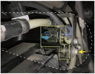
▶ Locate and install the solenoid valve as indicated
