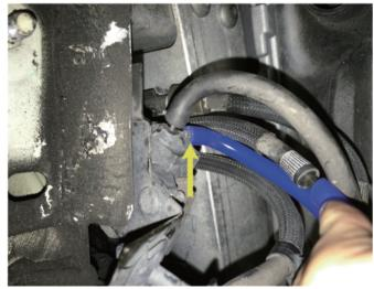
▶ Disconnect the original hose(out) and reconnect to Armytrix solenoid valve(in).
