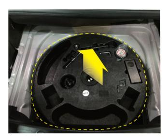
▶ Open the trunk. Remove the cover and find the point with black/blue wire as shown
