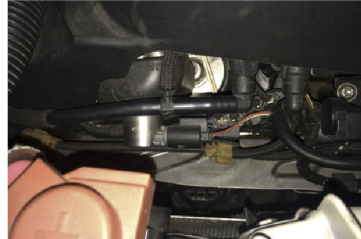
▶ Locate the source from vacuum pump
