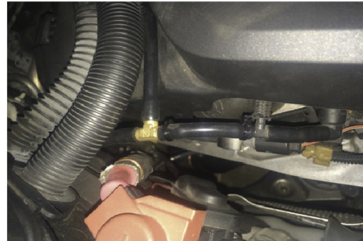
▶ Connect the Three way valve at the indicated point
