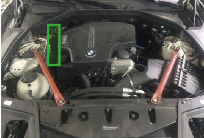
▶ The vacuum source is located on the left as indicated
