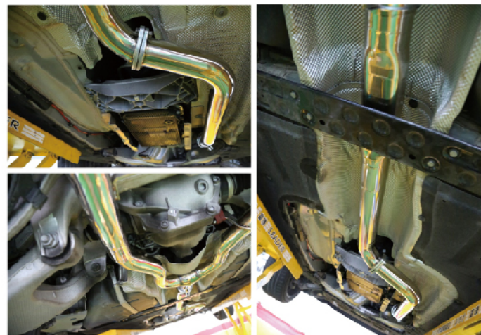
▶ 3. Install ARM L pipe, Mid-pipe and Y-pipe
