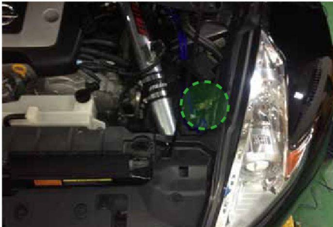
▶ Create a sole vacuum source with blue silicon tube
