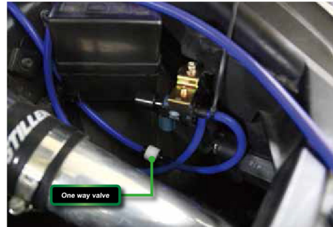
▶ After Connect blue silicon tube with solenoid valve, continue connect it with one-way-valve as red circle pointed
