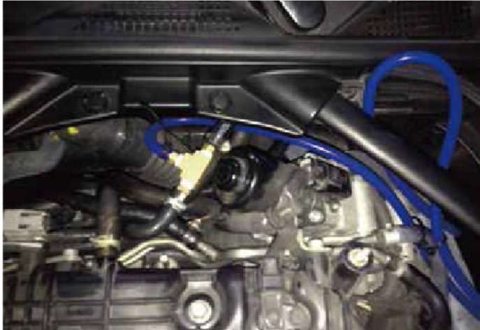
▶ Create a sole vacuum source with blue silicon tube
